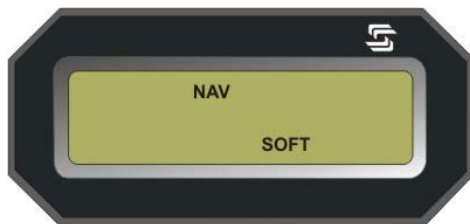
Fig. 3-5. Remote Annunciator Display, NAV Mode Engaged, SOFT Condition
