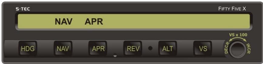
Fig. 3-32. AP Display, NAV APR Mode Engaged, Track LOC Front Course Inbound
