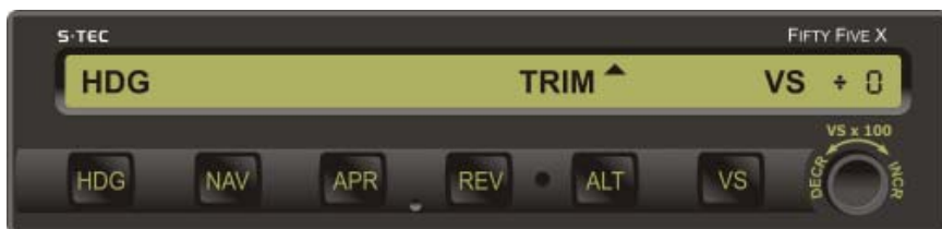
a. HDG and VS Modes Engaged, 0 FPM, TRIM UP Required
