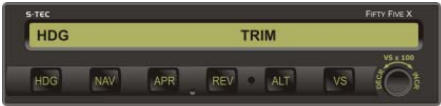
Fig. 3-16. AP Display, Manual Electric Trim in Progress
