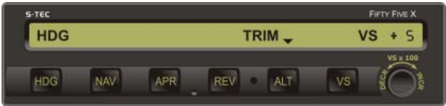
b. TRIM DN in Progress
