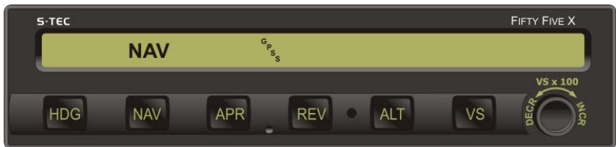
Fig. 3-9. AP Display, NAV GPSS Mode Engaged
