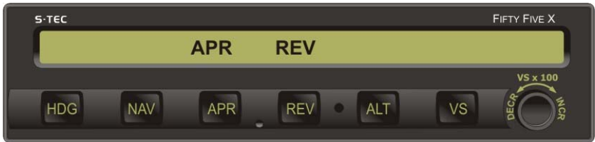
Fig. 3-31. AP Display, REV APR Mode Engaged, Track LOC Front Course Outbound
