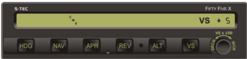
Fig. 3-13. AP Display, CWS Mode Engaged
