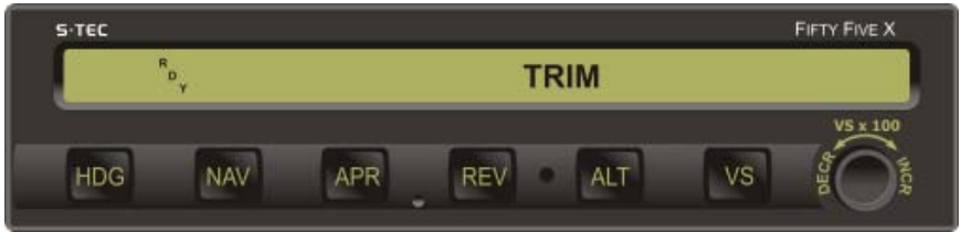
Fig. 2-15. AP Display, Manual Electric Trim in Progress (Pre-Flight)
