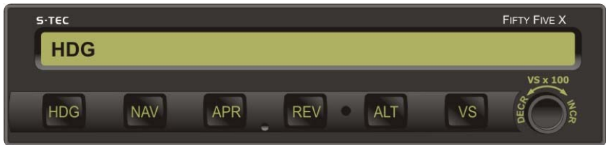
Fig. 3-1. AP Display, HDG Mode Engaged
