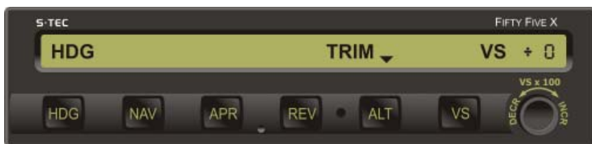
b. HDG and VS Modes Engaged, 0 FPM, TRIM DN Required
