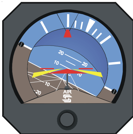
Fig. 3-39. FD Display, FD/AP Mode Engaged
