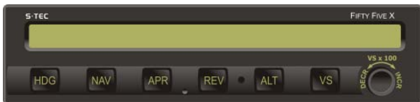
Fig. 2-5. AP Display, Turn Coordinator Failure
