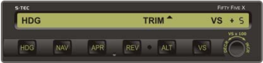
a. TRIM UP in Progress
